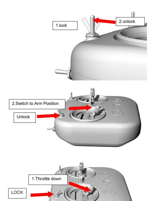
Unlocking refers to setting the Tinyhawk III Plus Freestyle into a flight-ready state. When the Tinyhawk III Plus Freestyle is first powered on, the propellers won't spin until it's unlocked.
