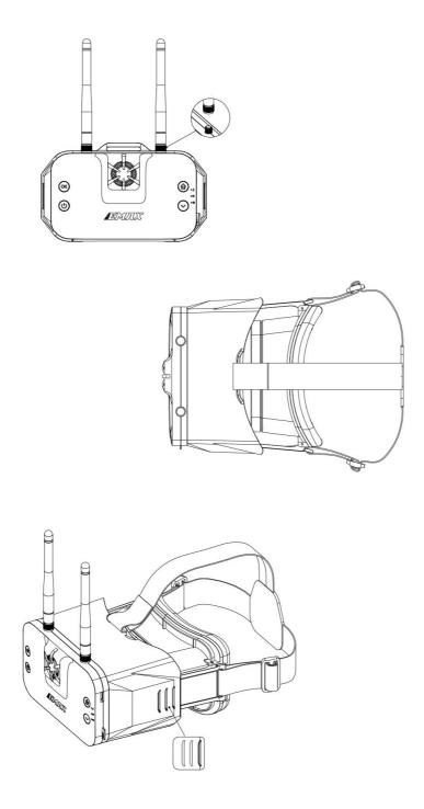
There are three distance adjustment slots, allowing for three different distances to be set. When adjusting, please ensure that the distance adjustment slots on the left and right sides are kept consistent.
