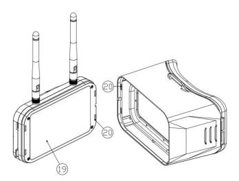
Flight goggles consist of two main components: the display module and the main body shell. These can be combined together using magnets or separated as needed.
