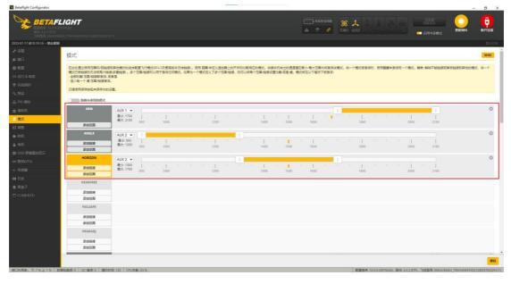
AUX 3 is a 2-position switch and is configured as the Flip Over After Crash mode.
