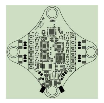
The Tinyhawk III Plus Freestyle's receiver is an onboard ELRS (2.4G) receiver. The RF module used is SX1280, employing SPI communication. It features a ceramic antenna (with a gain of 3dB) and operates within the frequency range of 2400-2480MHz. The receiver protocol used is CRSF, and its protocol version is ELRS V3.0.
